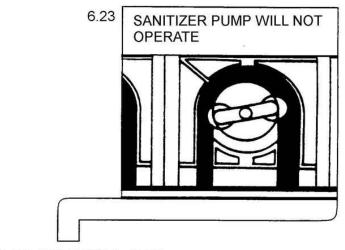
Is cam notch completely closed due to maladjustments?
