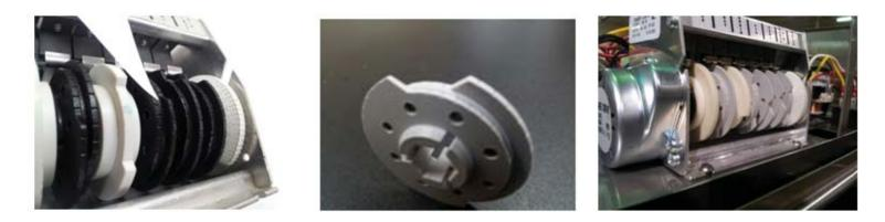
The arrow is pointed at the left-side wheel of the cam which is used to lengthen or shorten the low cam or the time ON for the respective switch. Adjustable cams are colored either black or gray.
