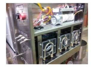
AFB prime switches and internal chemical pumps
