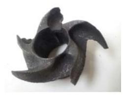
Impeller damaged from high acid solution
