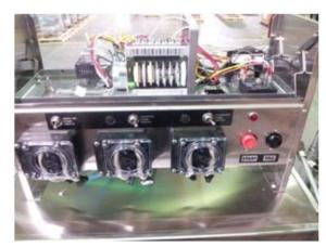
Showing control box, chemical pumps, prime switches
