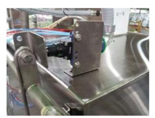
5-CD Door cut-off switch and lever arm
