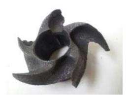
Impeller damaged from high acid solution
