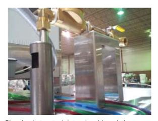
Showing hot water inlet, solenoid, and air gap
