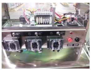
Showing control box, chemical pumps, prime switches
