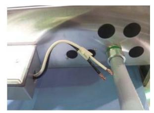
Showing power connection for 120v wiring
