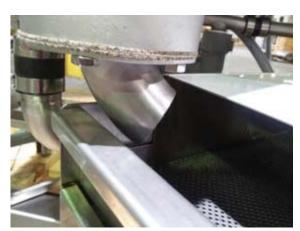
Correct alignment for sump to box
