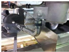
Single Pump, intake and discharge manifolds
